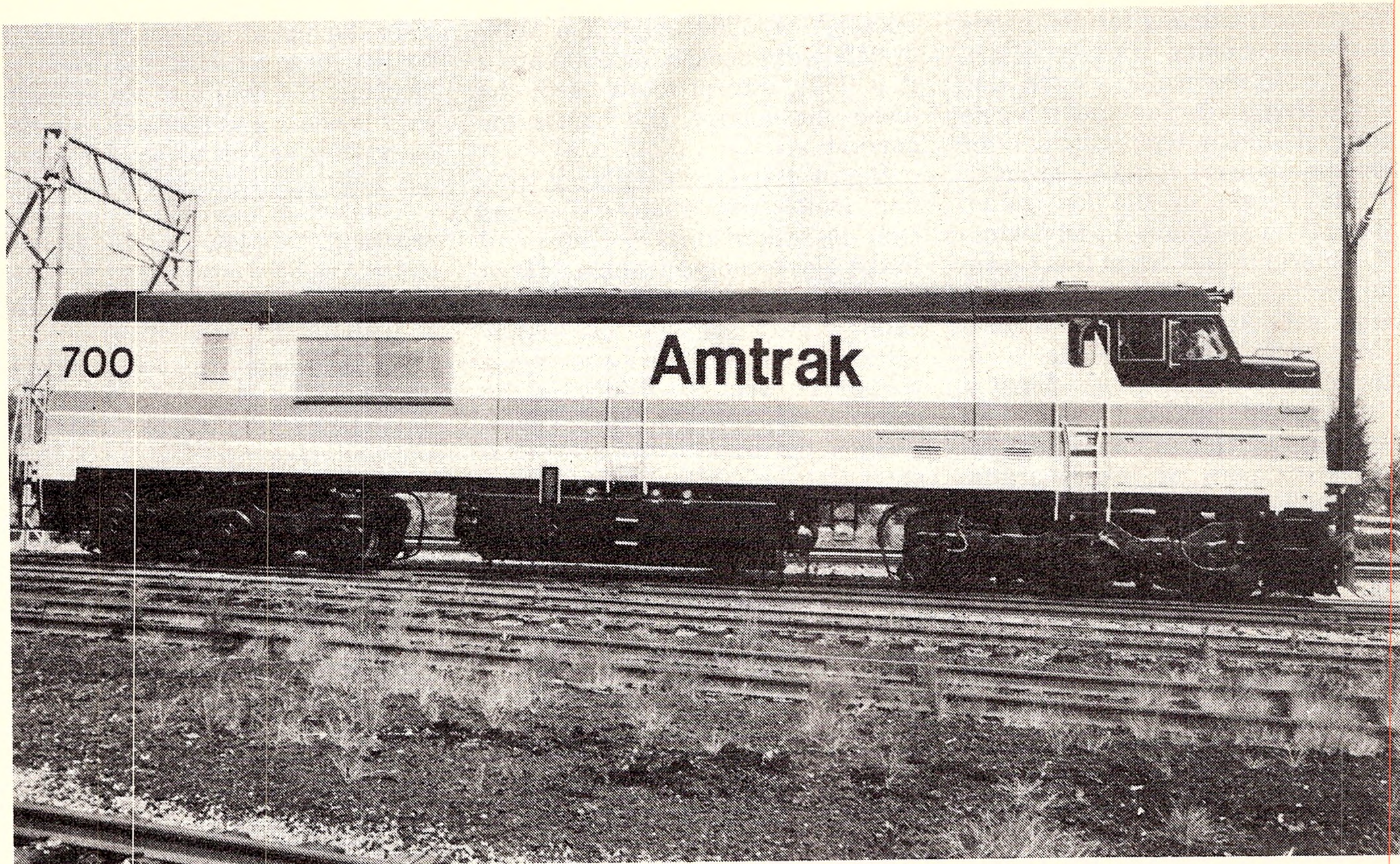
AMTRAK'S P30CH DIESEL-ELECTRIC locomotives feature a big 13,700 litre fuel tank for medium and long-haul operation. These 6-axle Co-Co locomotives are rated at 2.24MW and are geared for a maximum speed of 165km/hr.
