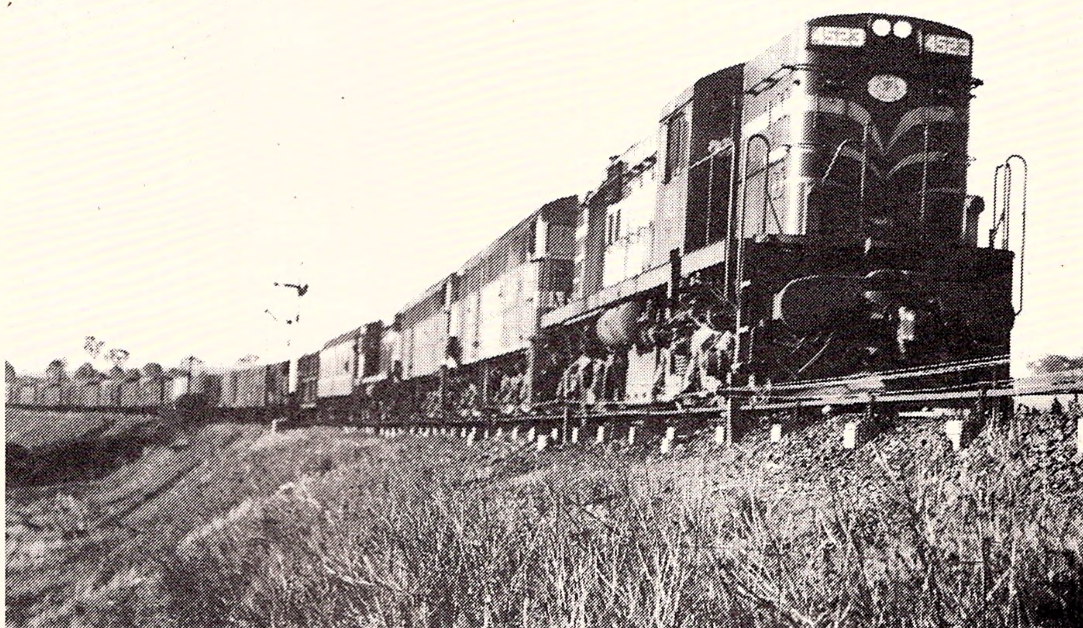
FOUR LOCOMOTIVES ARE used here on this NSW-SRA train to give a total power of 5.66MW. Leading is a 1.34MW 45 class locomotive weighing 112 tonnes. Next come two 1.49MW 442 class locomotives, each weighing 115 tonnes. The fourth locomotive is another 45 class.
