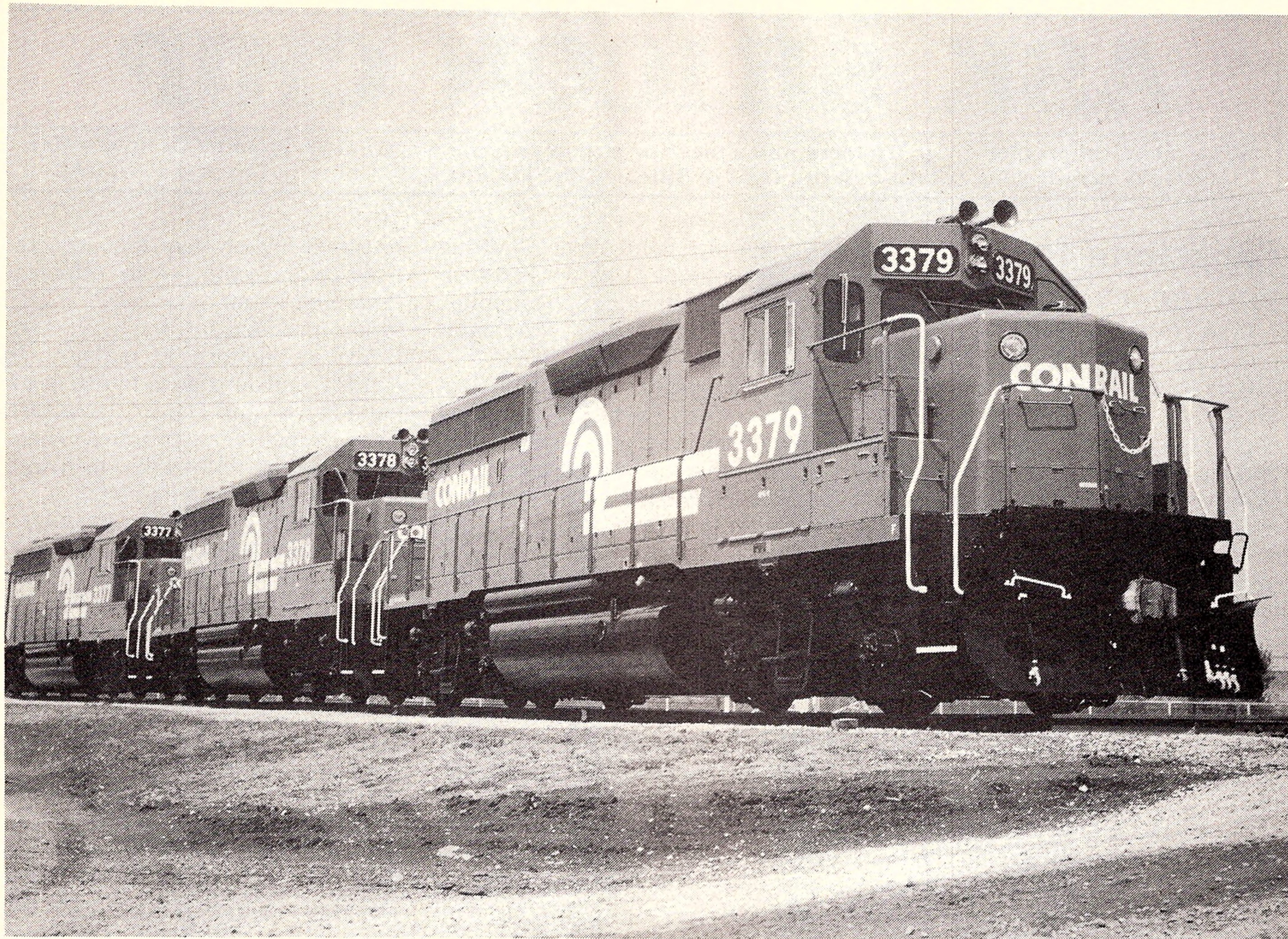
AMERICAN MUSCLE — THREE NEW GP40 diesel-electric locomotives on their way to Conrail (USA) from the General Motors Electro-Motive Division. These 2.24MW (3000hp) Bo-Bo locomotives are used for general service.
