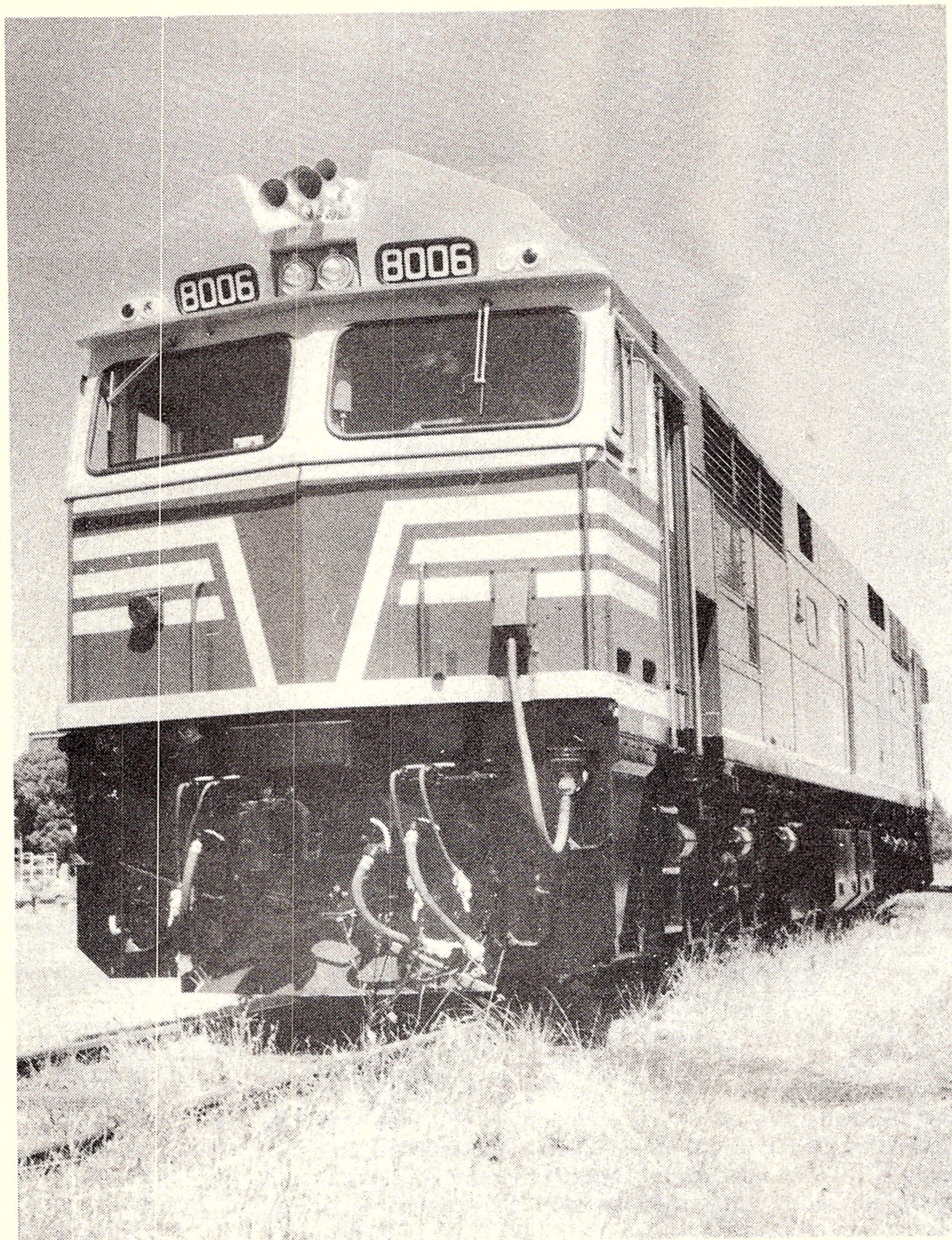
THE NSW-SRA 80-CLASS diesel-electric locomotive is rated at 1.492MW (2000hp), weighs 119 tonnes, and is capable of express speeds up to 130km/hr. The first unit was built by Comeng for the SRA in December 1978.
